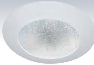
Ingress of Moisture
