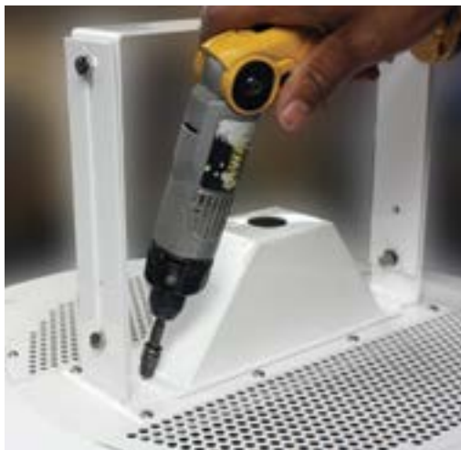
1. Remove the two (2) nuts holding the cover.
