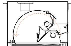
The ambient lamp assembly rotates forward for easy access when relamping.
