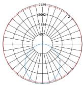
$\label{eq:max-cond} \text{Max Candela} = 2789 \text{ Located At Horizontal Angle} = 15, \text{Vertical Angle} = 5$
