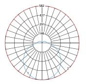
Max Candela = 582 Located At Horizontal Angle = 0, Vertical Angle = 0 — 1 - Vertical Plane Through Horizontal Angles (0-180) (Through Max. Cd.) — 2 - Horizontal Cone Through Vertical Angle (0) (Through Max. Cd.)
