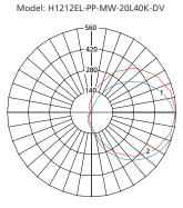
Max Candela = 560 Located At Horizontal Angle = 0, Vertical Angle = 80 1 - Vertical Plane Through Horizontal Angles (0-180) (Through Max. Cd.) 2 - Horizontal Cone Through Vertical Angle (80) (Through Max. Cd.) Model: H1212FL-PP-MW-20L40K-DV
