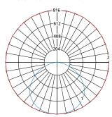
$\mbox{Max Candela} = 816 \mbox{ Located At Horizontal Angle} = 0, \mbox{Vertical Angle} = 0$
