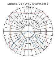
Max Candela = 8326 Located At Horizontal Angle = 45, Vertical Angle = 42.5 1 - Vertical Plane Through Horizontal Angles (45 - 225) (Through Max. Cd.) 2 - Horizontal Cone Through Vertical Angle (42.5) (Through Max. Cd.)
