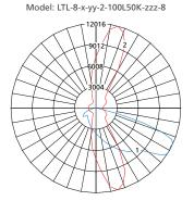
Max Candela = 12016 Located At Horizontal Angle = 75, Vertical Angle = 57.5 1 - Vertical Plane Through Horizontal Angles (75 - 255) (Through Max. Cd.) 2 - Horizontal Cone Through Vertical Angle (57.5) (Through Max. Cd.)
