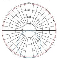
$Maximum\ Candela = 1628\ Located\ At\ Horizontal\ Angle = 15, Vertical\ Angle = 5$
