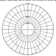
Maximum Candela = 1761 Located At Horizontal Angle = 15, Vertical Angle = 5
