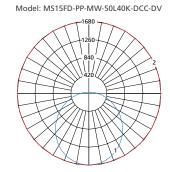
Max Candela = 1680 Located At Horizontal Angle = 0, Vertical Angle = 0 — 1 - Vertical Plane Through Horizontal Angles (0-180) (Through Max. Cd.) 2 - Horizontal Cone Through Vertical Angle (0) (Through Max. Cd.)
