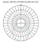
Max Candela = 1006 Located At Horizontal Angle = 0, Vertical Angle = 0 1 - Vertical Plane Through Horizontal Angles (0-180) (Through Max. Cd.) 2 - Horizontal Cone Through Vertical Angle (0) (Through Max. Cd.) Model: MS15EL-PP-MW-25L40K-DCC-DV
