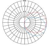
Max Candela = 950 Located At Horizontal Angle = 0, Vertical Angle = 65 — 1 - Vertical Plane Through Horizontal Angles (0-180) (Through Max. Cd.) — 2 - Horizontal Cone Through Vertical Angle (65) (Through Max. Cd.)
