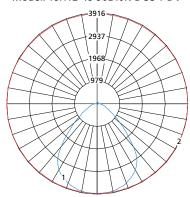
Maximum Candela = 3916 Located At Horizontal Angle = 75, Vertical Angle = 2.5
