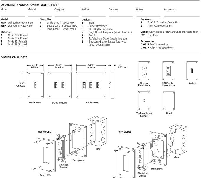
For Steel or Block Wall Construction
